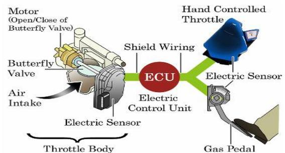
Fig. 2 System Schematic Diagram
